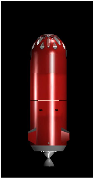
balloon which lifts the rocket to altitude before the rocket engines are fired. Guidance is accomplished using an integrated GPS / INS system into the RCS (Reaction Control System). The vehicle is a cylindrical rocket with a blunt nose cone, and uses inflatable base cushions for both the capsule and propulsion sections that land separately (used to cushion the landing). *Wild Fire MKVI* is approximately 8
